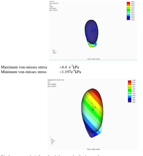
Displacement analysis for safety helmet made of polypropylene Maximum Displacement =23.5268mm Minimum Displacement =1.64667mm
