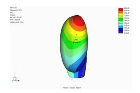
Displacement analysis of the safety helmet made of banana fiber and coir Maximum Displacement  $=6.89 e^{-2}$ mm Minimum Displacement  $=4.148e^{-2}$ mm
